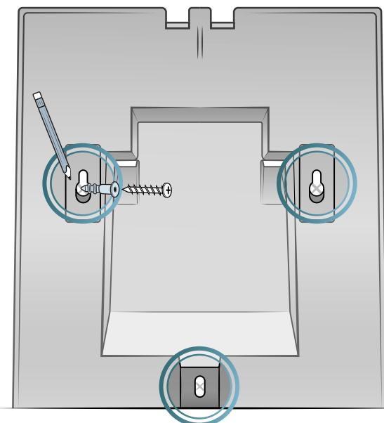
mounting height is 55" from floor to bottom of bracket (**Figure 2**).
