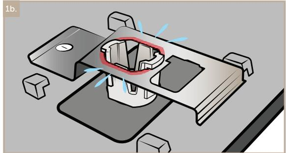
2. Slide lock cover back into place if removed.
