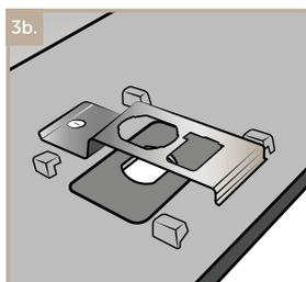
3. Support lock assembly from underneath with hand. Use a flathead screwdriver to remove retaining clip. Lock may fall into hand.
