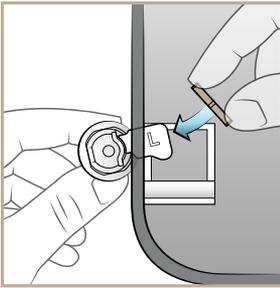
1. Insert the Left Push Button tab through the cover opening, and thread Lock Nut over tab.
