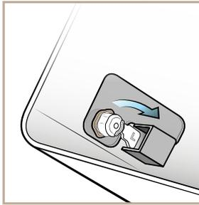
2. Position tab into the pocket of the locking latch.
