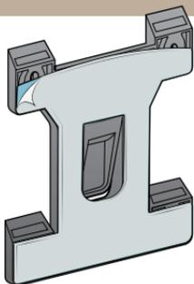
1. Open and remove bracket. Ensure that bottom edge of bracket is a minimum 15  $\frac{3}{16}$ " (396mm) above any surface.
